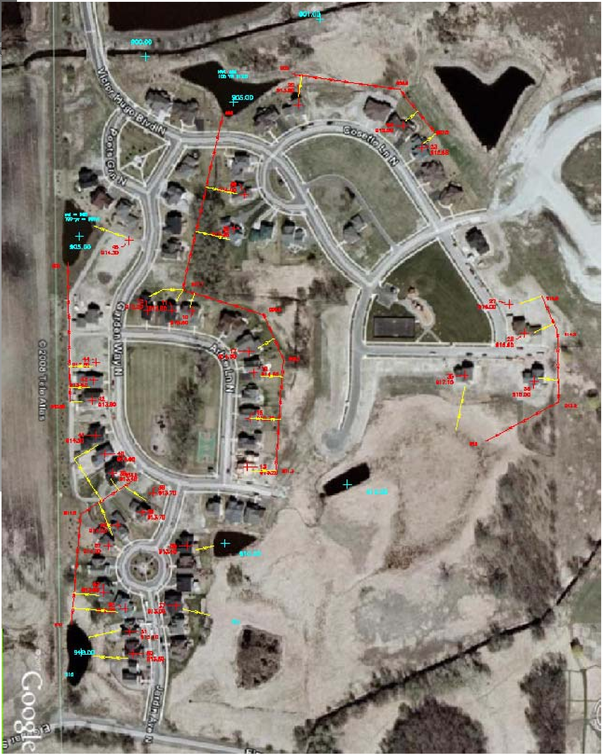
Figure 4 – Diagram of foundation-drainage system proposed for the Victor Gardens Development, Hugo, MN
